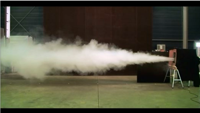
Figure 2. Air flow: 110 m 3 /h Number of nozzles: 2 Horizontal air discharge
