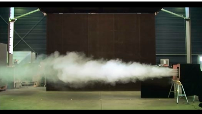
Figure 4. Air flow: 110 m 3 /h Number of nozzles: 4 Horizontal air discharge
