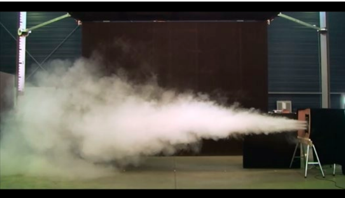
Figure 3. Air flow: 110 m 3 /h Number of nozzles: 3 Horizontal air discharge
