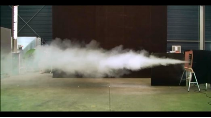
Figure 1. Air flow: 110 m 3 /h Number of nozzles: 1 Horizontal air discharge
